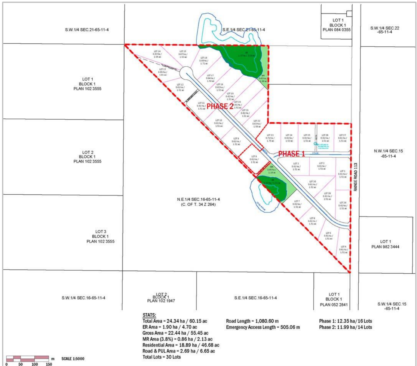
Figure 3.4. Proposed development area (outline in red) concept plan within Lac La Biche County, Alberta in NE16-65-11-W4M (Reproduced from Select Engineering Consultants - March 2, 2022; – Concept Option 7).
