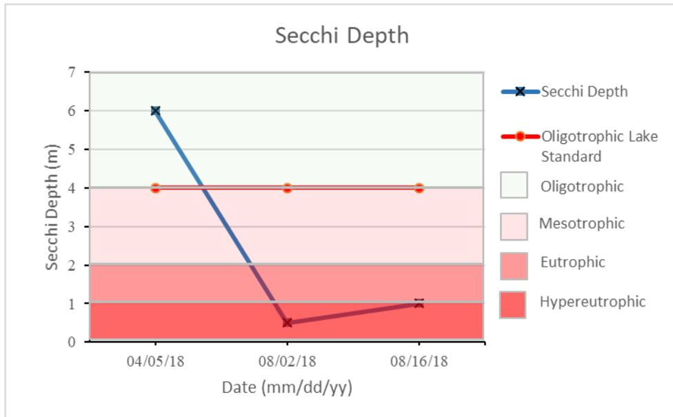
Figure 2: Secchi depths measured in Fork Lake – 2018
