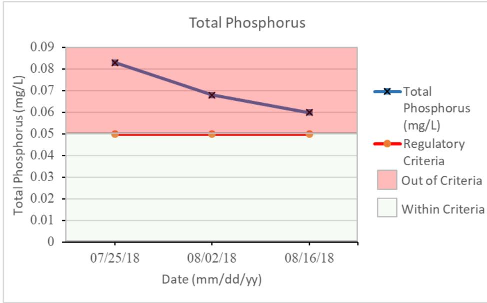
Figure 7: Total phosphorus in composite samples of Fork Lake - 2018
